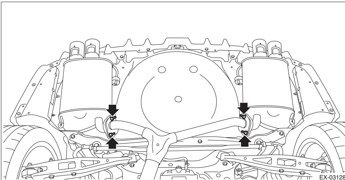
4) Install the bolts, springs, and nuts which secure the center exhaust pipe (rear) to the rear exhaust pipe.
